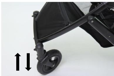
To lock the swivel on the front wheels, slide the lever downwards.
